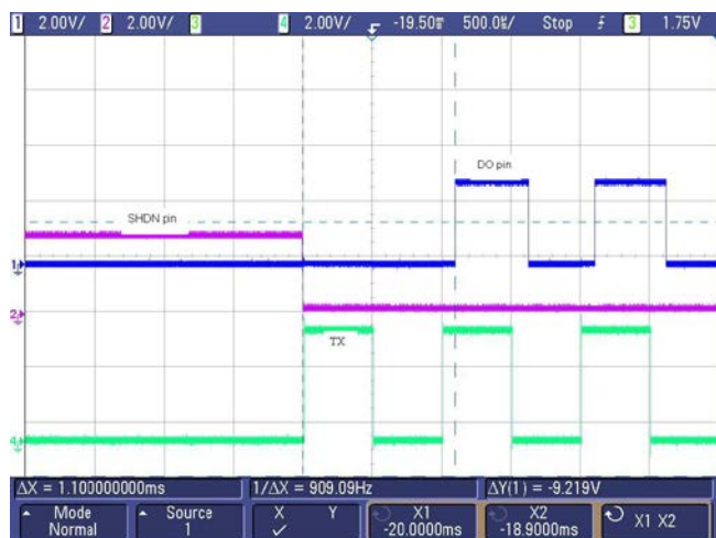
Figure 10. Time-to-Preamble Data after Shut Down Cycle, Room Temperature
