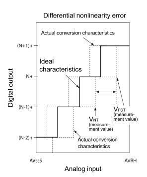
Nonlinearity error of digital output N =  $\frac{V_{NT} - \{1LSB \times (N-1) + V_{OT}\}}{1LSB}$  [LSB]
