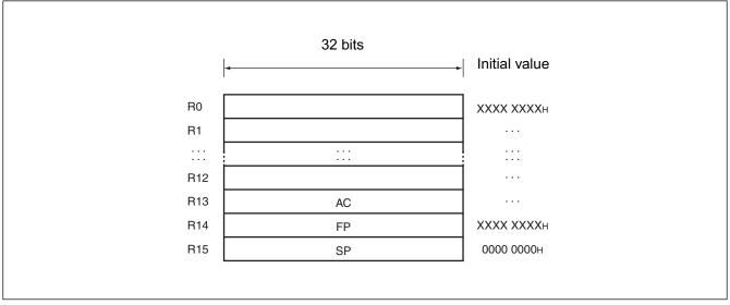
Registers R0 to R15 are general-purpose registers. These registers can be used as accumulators for computation operations and as pointers for memory access.
