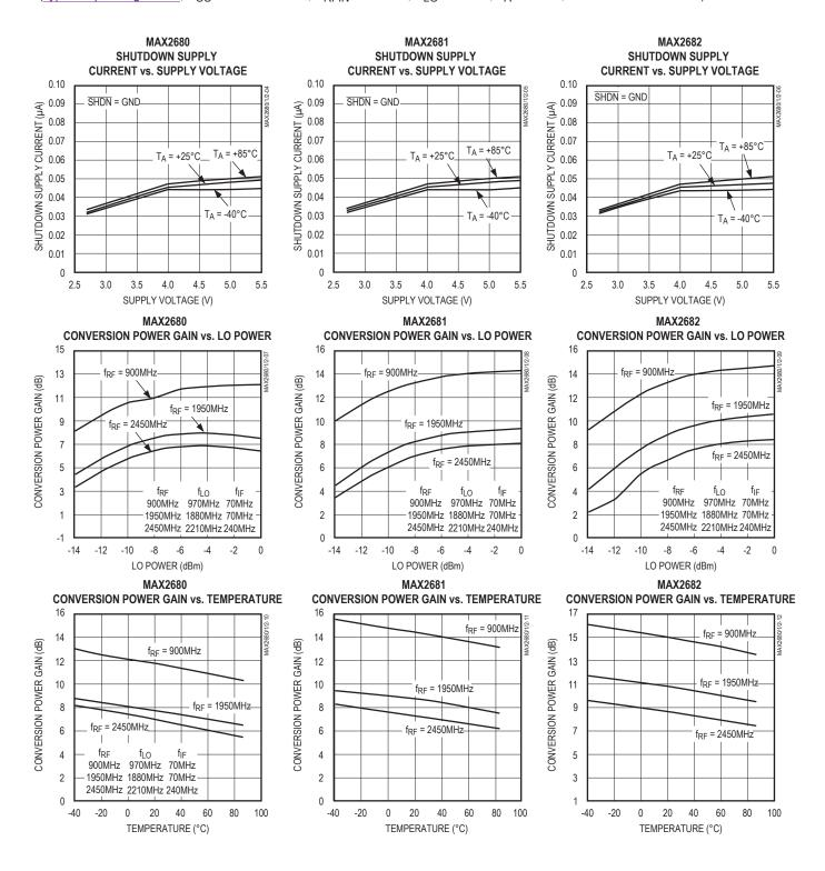
(Typical Operating Circuit, V<sub>CC</sub> = SHDN = +3.0V, P<sub>RFIN</sub> = -25dBm, P<sub>LO</sub> = -5dBm, T<sub>A</sub> = +25°C, unless otherwise noted.)
