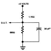
\*INCLUDING SCOPE AND JIG CAPACITANCE
