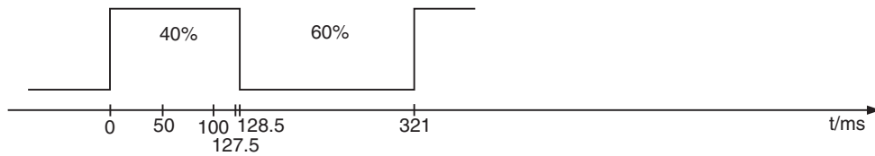
Figure 11-2. Application 1: 12V Version, Turn Signal Switches to GND, Hazard Switch to GND
