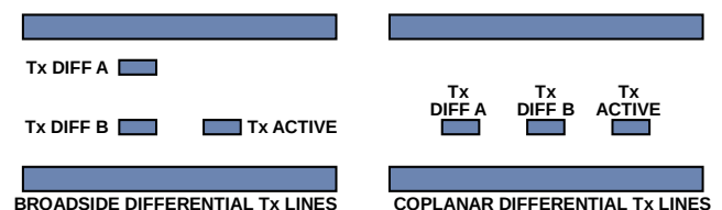
Figure 66. Broadside vs. Coplanar Differential Stripline Routing Techniques
