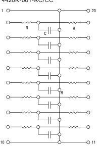
These low-pass filters are ideal for installation between I/O drivers and RS 232 connectors.
