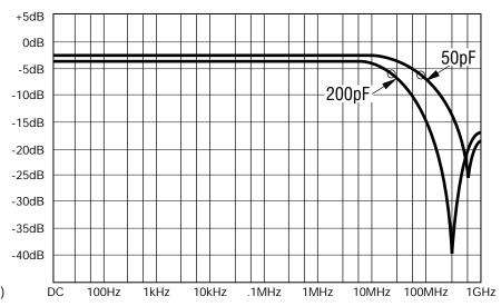
O indicates - 3dB rolloff frequency (f<sub>C</sub>)
