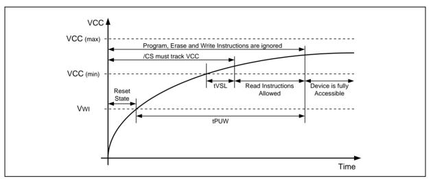
Figure 58a. Power-up Timing and Voltage Levels
