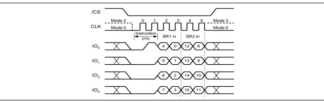
Figure 9d. Write Status Register-1/2 Instruction (QPI Mode)
