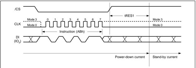
Figure 38a. Release Power-down Instruction (SPI Mode)
