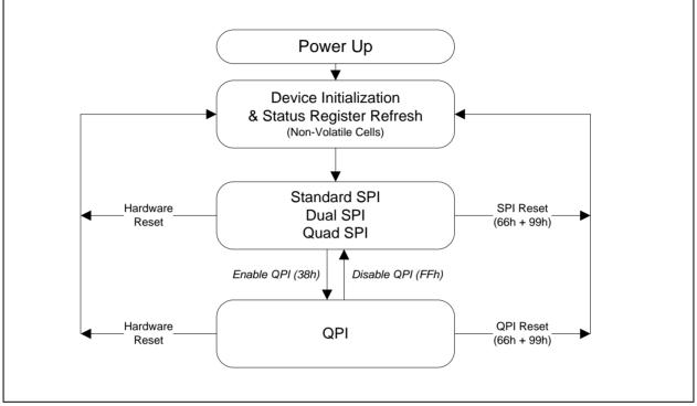
Figure 3. W25Q128JV Serial Flash Memory Operation Diagram
