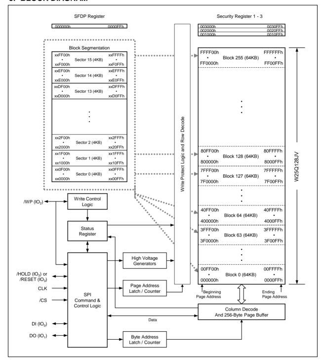
Figure 2. W25Q128JV Serial Flash Memory Block Diagram
