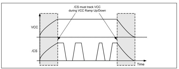
Figure 58b. Power-up, Power-Down Requirement
