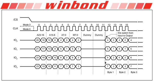
Figure 24b. Fast Read Quad I/O Instruction (Previous instruction set M5-4 = 10, SPI Mode)
