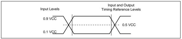
Figure 59. AC Measurement I/O Waveform
