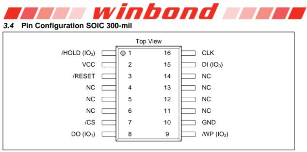
Figure 1c. W25Q128JV Pin Assignments, 16-pin SOIC 300-mil (Package Code F)
