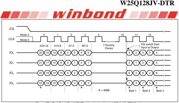
Figure 27b. Fast Read Quad I/O (Previous instruction set M5-4=10, SPI Mode)
