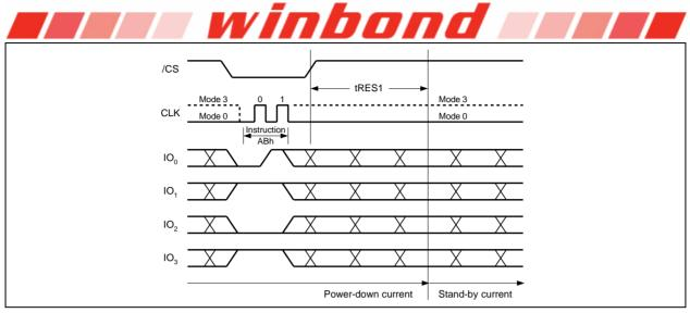
Figure 38b. Release Power-down Instruction (QPI Mode)
