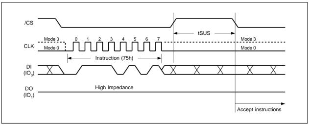
Figure 35a. Erase/Program Suspend Instruction (SPI Mode)
