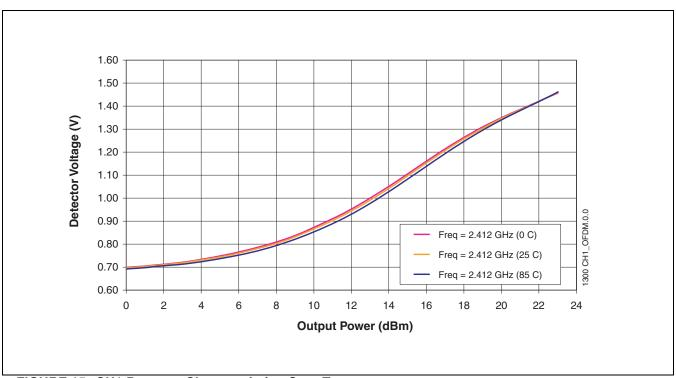
FIGURE 15: CH1 Detector Characteristics Over Temperature
