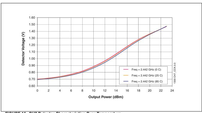
FIGURE 16: CH7 Detector Characteristics Over Temperature
