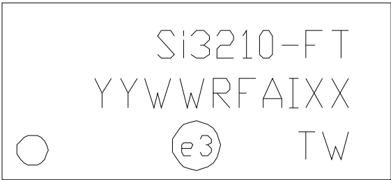
Figure 40. TSSOP Top Mark Diagram
