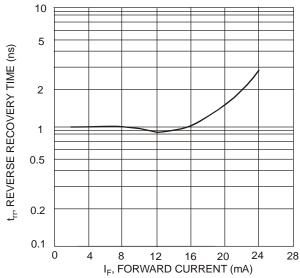
Fig. 4 Typical Reverse Recovery Time Characteristics
