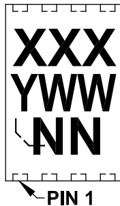
8-Lead DFN (2x3x0.9 mm)
