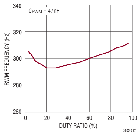
PWM Signal Generator Frequency vs Duty Ratio
