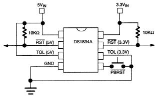
Note: If outputs are pulled-up to different voltages the outputs can not be connected to form a wired "AND".
