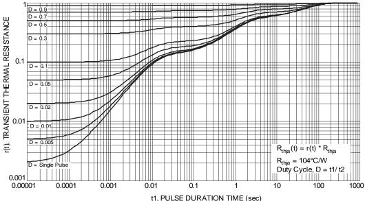
t1, PULSE DURATION TIME (sec) Figure 13 Transient Thermal Resistance
