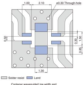
Coplanar waveguide(Line width and Gap of Line to GND) be designed to match 50\Omega characteristic impedance, depending on PCB material and thickness.
