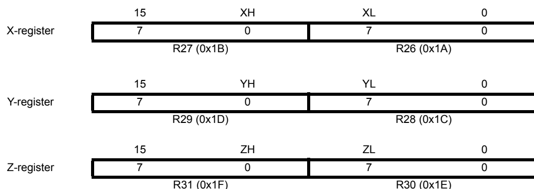
Figure 5-3. The X-, Y-, and Z-registers
