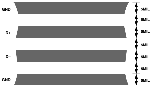
Figure 16. Typical Arrangement of Signal Tracks
