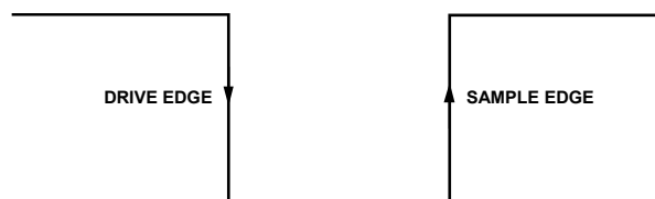
Figure 78. SPI Mode 0 SCLK Edges
