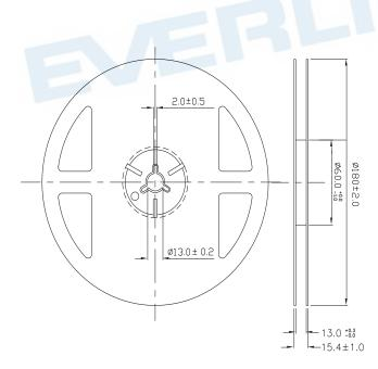
Note: The tolerances unless mentioned are ±0.1, unit=mm
