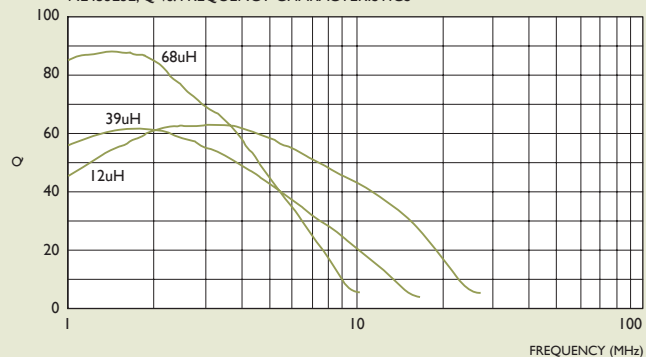
NL453232, Q vs. FREQUENCY CHARACTERISTICS
