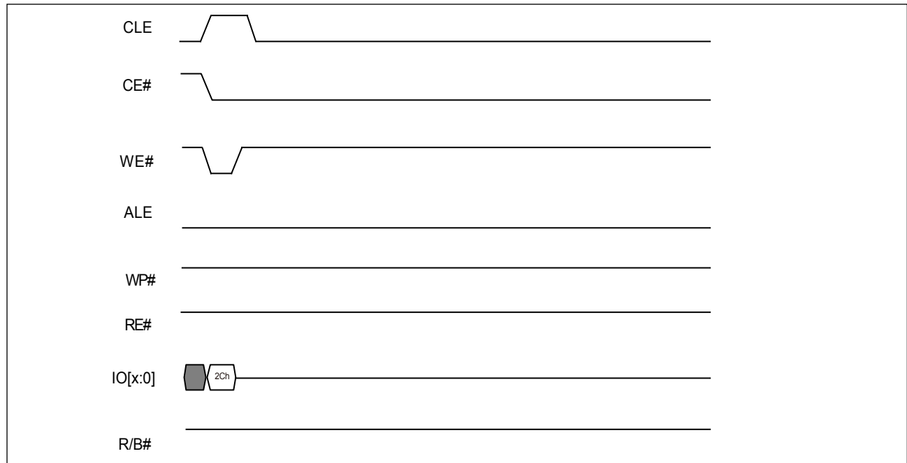
Figure 40. AC Waveforms for Block Solid-Protect
