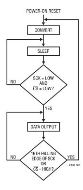
Figure 2. LTC2450-1 State Transition Diagram
