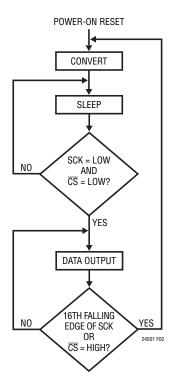
Figure 2. LTC2450-1 State Transition Diagram
