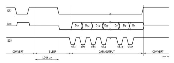
Figure 5. Idle-High (CPOL = 1) Serial Clock Operation Example. The Rising Edge of CS Starts a New Conversion
