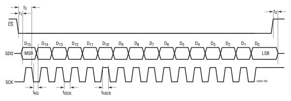
Figure 3. Data Output Timing
