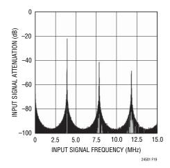
Figure 19. Input Signal Attenuation vs Frequency
