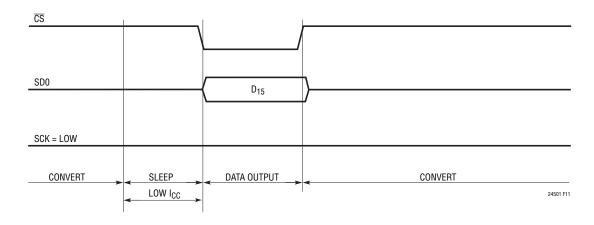
Figure 11. Idle-Low (CPOL = 0) Clock and Minimum Data Output Length Example
