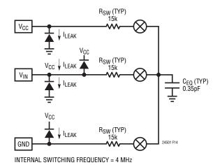
Figure 14. LTC2450-1 Analog Pins Equivalent Circuit
