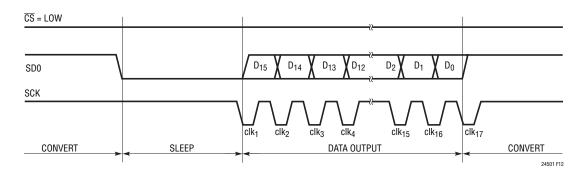
Figure 12. 2-Wire, Idle-High (CPOL = 1) Serial Clock, Operation Example
