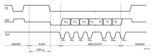
Figure 6. Idle-High (CPOL = 1) Clock Operation Example.
