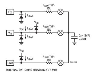
Figure 14. LTC2450-1 Analog Pins Equivalent Circuit
