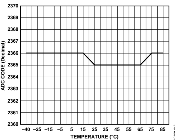
Figure 18. ADC Code vs. Temperature (Fixed Analog Input)
