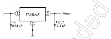
Be sure to connect a capacitor near the input terminal and output terminal between both terminals and GND. The capacitances should be determined experimentally. In particular, adequate investigation should be made so that there is no problem even in high or low temperatures.
