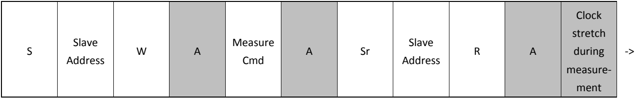
Sequence to perform a measurement and read back result (Hold Master Mode)
