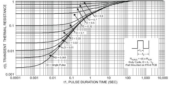
Fig. 9 Transient Thermal Resistance
