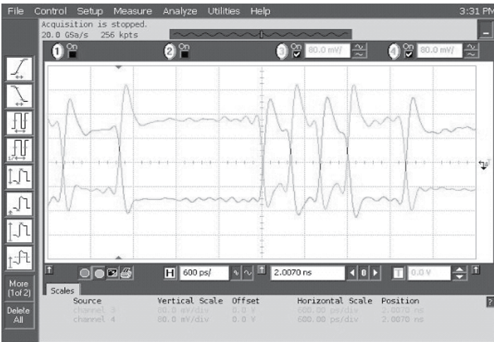
Data Waveforms, 3.0Gbps (left) & 6.0Gbps (right)
