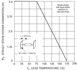
Fig. 5, Steady State Power Derating
