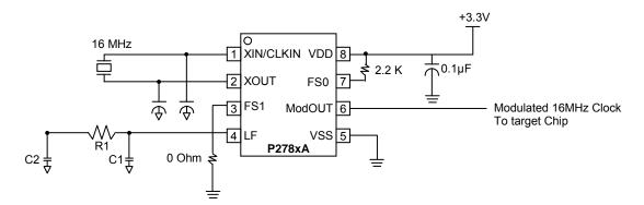
Note: Both logic input pins FS1 and FS0 have to be connected to either VDD or VSS. Do not leave them floating.
