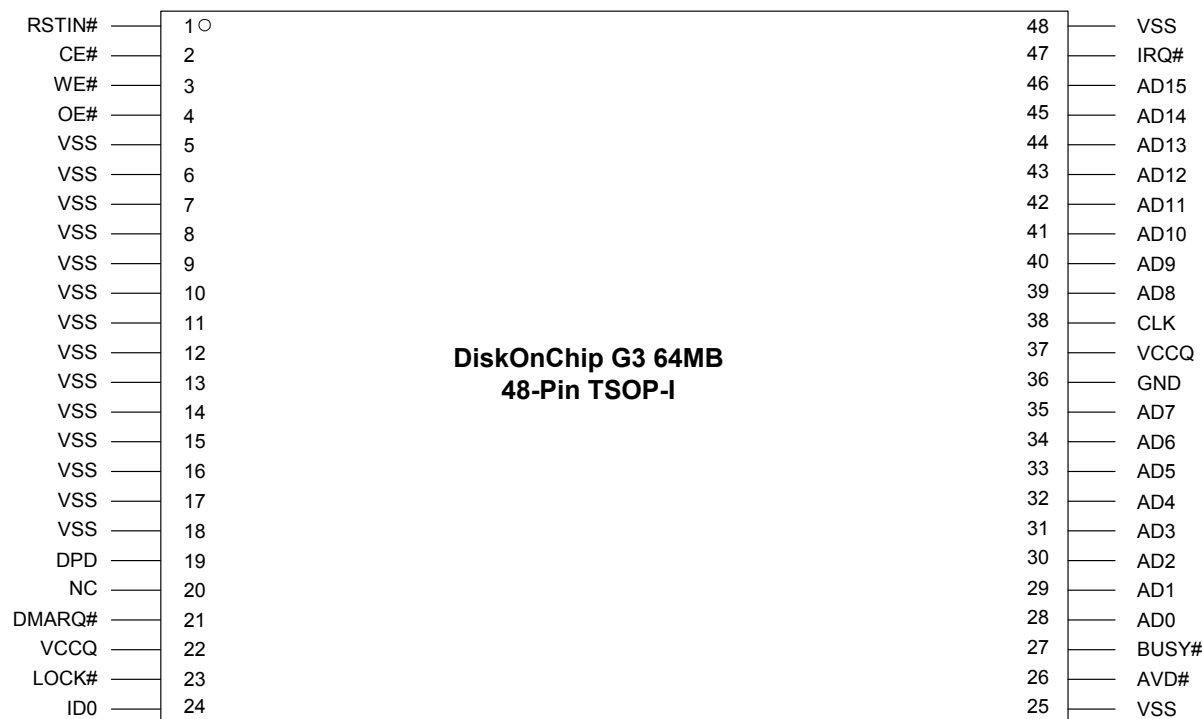
Figure 6: Pinout for Multiplexed Interface (DiskOnChip 64MB/512Mb TSOP-I Package)
