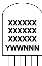
6-Lead DFN (2x2x0.9 mm)
