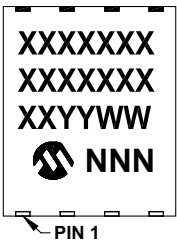
8-Lead DFN-S (6x5x0.9 mm)
