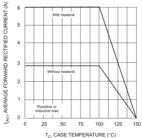
Fig. 1 Forward Current Derating Curve
