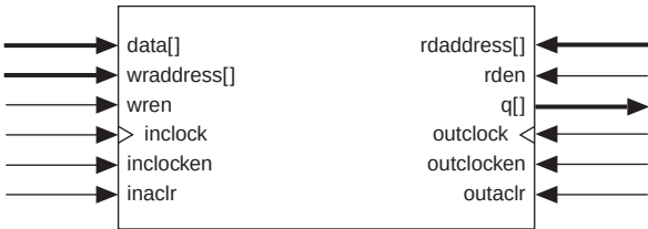
Figure 2–13. Simple Dual-Port & Single-Port Memory Configurations
