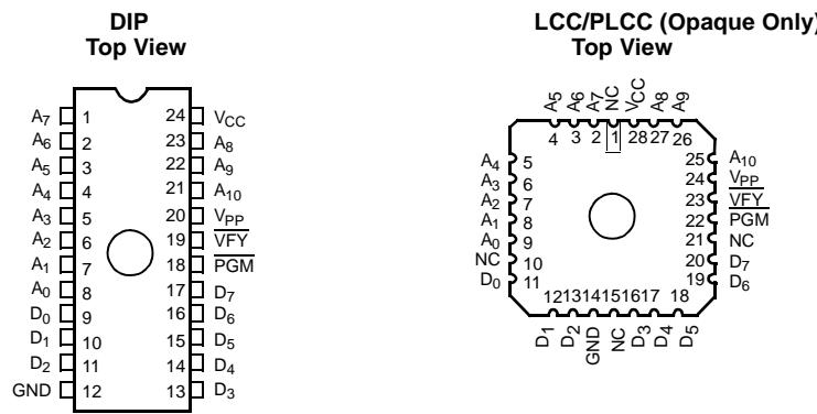
**Figure 1. Programming Pinouts**
