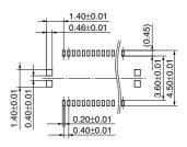
Recommended metal mask pattern Metal mask thickness: Here, 120 μm (Terminal portion opening area ratio: 66%) (Metal portion opening area ratio: 100%)
