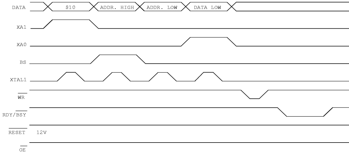
Figure 63. Programming the Flash Waveforms
