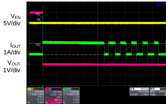
Output Short to GND Current ( V_{IN} = 5V , C_{IN} = 1.0\mu F )
