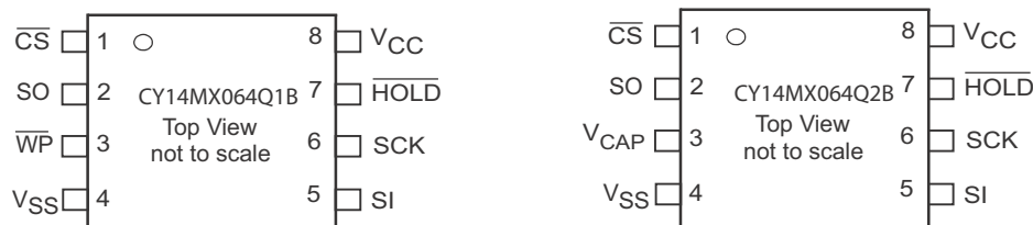
Figure 1. 8-pin SOIC pinout [1, 2]
