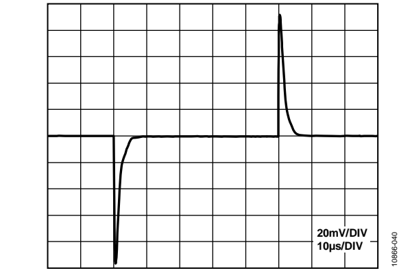
Figure 40. Reference Buffer Load Transient Response (100 \mu A Load Change)
