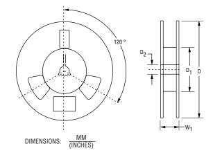
Devices are packed in accordance with EIA 481 standard specifications shown here.
