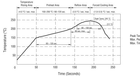
Peak Temperature: 245 °C max. Max. Peak Temperature: -5 °C, 30 sec. max. Max. Time Above 217 °C: 60 ~ 150 sec. max.
