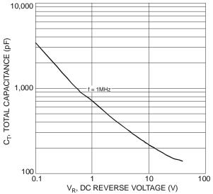
Fig. 4 Total Capacitance vs. Reverse Voltage
