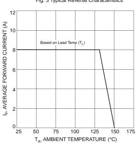
Fig. 5 Forward Current Derating Curve
