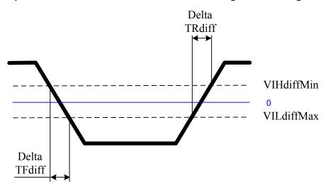
**AC and DC Output Measurement Levels**
