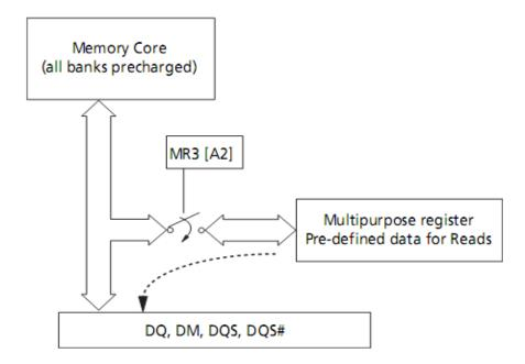
Fig. 1: MPR Block Diagram
