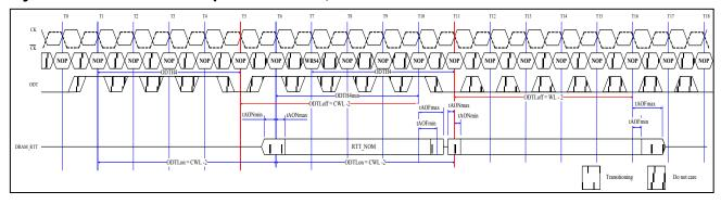
ODT must be held for at least ODTH4 after assertion (T1); ODT must be kept high ODTH4 (BL=4) or ODTH8 (BL=8) after Write command (T7). ODTH is measured from ODT first registered high to ODT first registered low, or from registration of Write command with ODT high to ODT registered low. Note that although ODTH4 is satisfied from ODT registered at T6 ODT must not go low before T11 as ODTH4 must also be satisfied from the registration of the Write command at T7.
