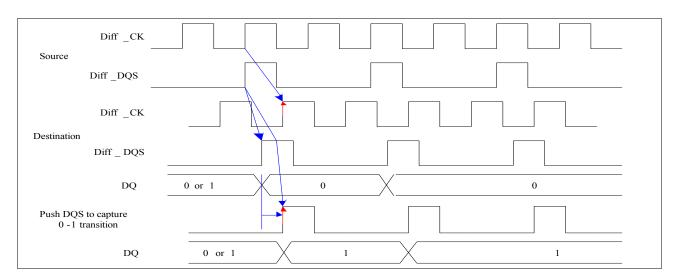
DQS/DQS driven by the controller during leveling mode must be determined by the DRAM based on ranks populated. Similarly, the DQ bus driven by the DRAM must also be terminated at the controller.
