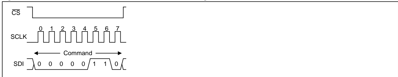
Figure 4-4. SPI Write Enable Transaction Functional Timing
