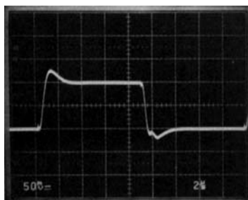
Small-Signal Transient Response, Pin 1 = V -
