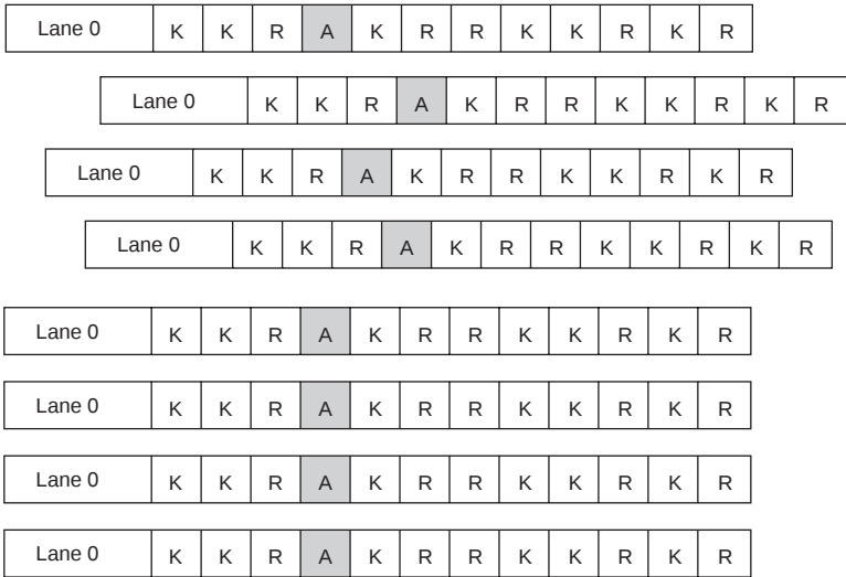
Figure 2–19. Before & After the Channel Aligner
