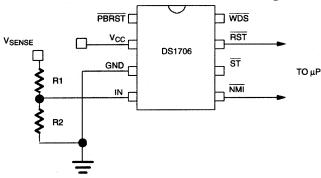
$$V_{SENSE} = \frac{R1 + R2}{R2} \times 1.25 \qquad V_{MAX} = \frac{V_{SENSE}}{V_{TP}} \times V_{CC}$$
