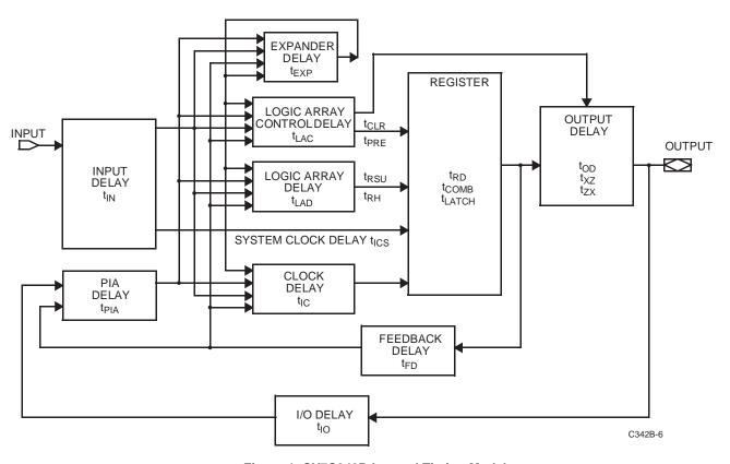
Figure 1. CY7C342B Internal Timing Model
